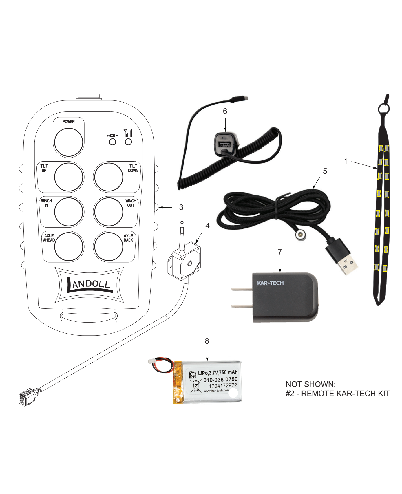
Figure 9-35: Remote Control Assembly, Wireless, Kar-Tech (Before 08/01/2019)
