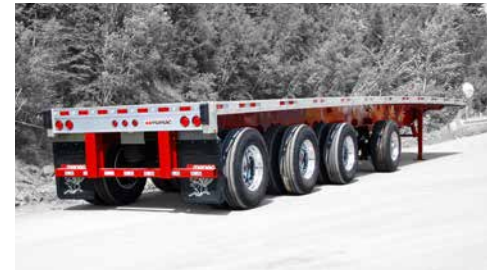
60,000 lb. capacity coil package
